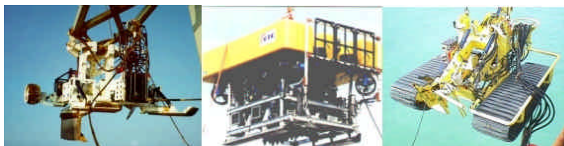
Figure 4 : A cable plough, trenching ROV and seabed tractor
