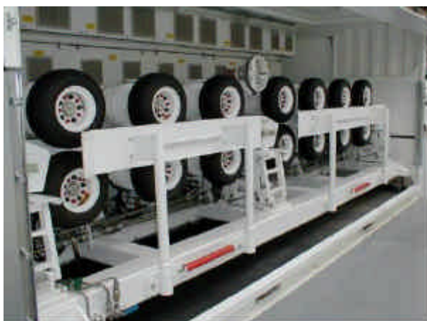
Figure 3 : A 7 Wheel Pair Linear Cable Engine
