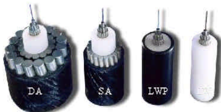
Figure 2 : Cable Armouring (DA, SA, LWP, LW)
